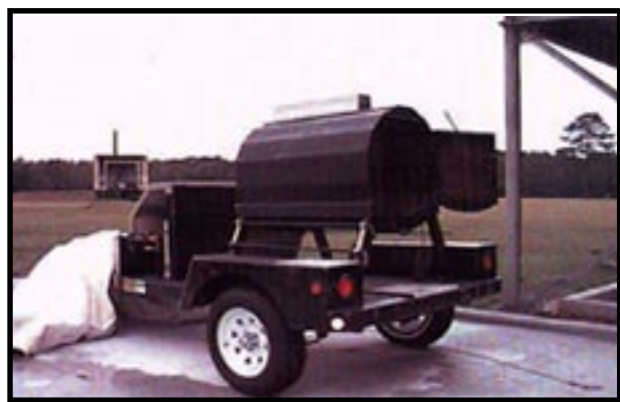
View of Hurd Burn Unit. This is a mobile unit which can be used for treating small quantities of PEP.
